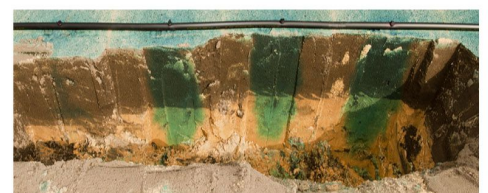
The second photo is from research carried out by the West Australian Department of Primary Industries and Regional Development to 'show water movement below drip irrigation'.
