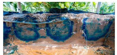
The first photo is from research carried out by Michigan State University to determine 'Drip Irrigation Water Distribution Demonstration' of sub surface drip line layer at different depths. This shows that there is an absence of lateral water spread beneath the surface.
